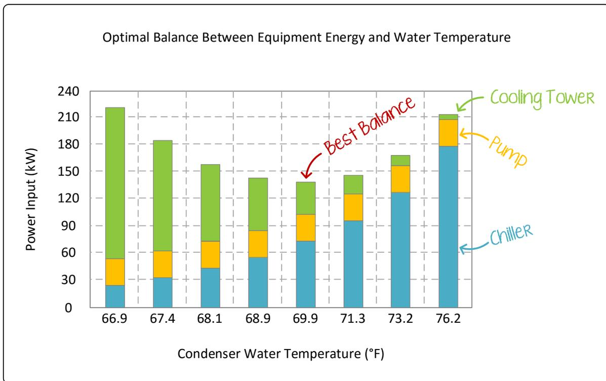
The above chart shows simulation calculations indicating that the optimal balance between chiller, pump, and tower energy occurs at a cooling tower water setpoint of 69.9°F with a pump flow rate of 66% of chiller design. This simulation method is not power demand, delta-T, or adaptive-based; rather it performs its optimized search using public domain equipment performance models and requires no information from the chiller to operate.
